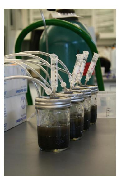
Figure 3 – Helium flushing during DEA
