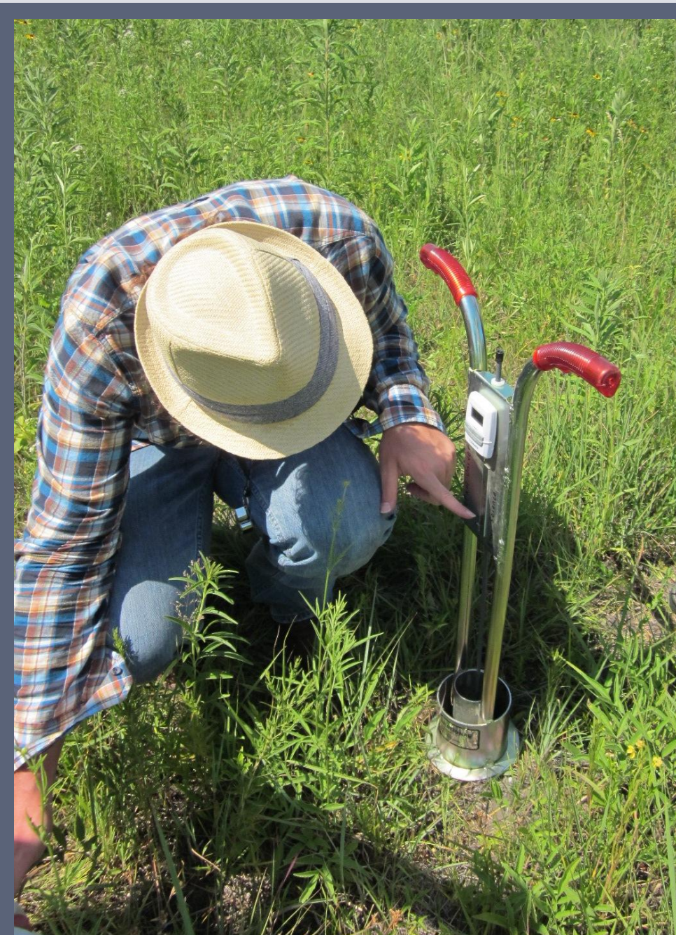
Figure 2: Infiltrator used to measure rate water infiltrates into soil
