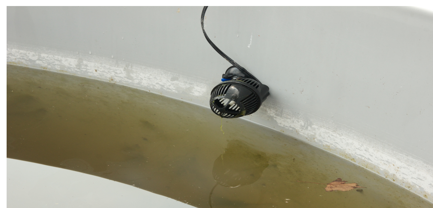
Fig. 3. Water pump attached to the side of a mesocosm used to simulate river flow
