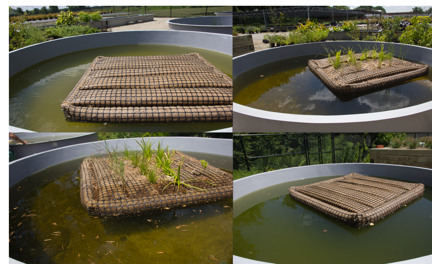
Fig. 1. All four mesocosms 6 weeks after initial planting. Noticeable differences in turbidity levels between unplanted and planted treatments
